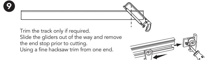
Trim the track only if required. Slide the gliders out of the way and remove the end stop prior to cutting. Using a fine hacksaw trim from one end.
