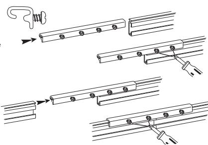
**B** Slide the second track into the joiner. Secure in place with screws provided.
