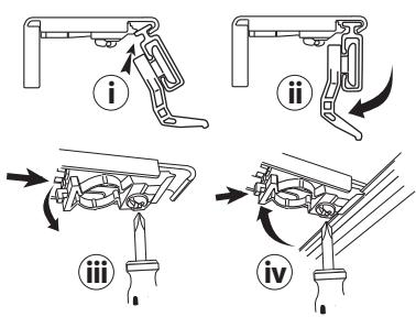
**NOTE:** For bay returns with top fix we recommend fixing the supports to the track prior to hanging
