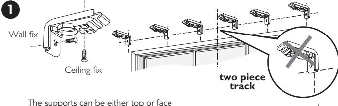
The supports can be either top or face fixed. Evenly space the supports along the window length making sure they are level. For 2 piece tracks using a joiner - do not place a support at the centre where the two tracks will join.
