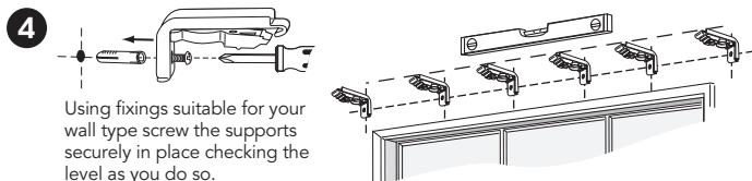
Using fixings suitable for your wall type screw the supports securely in place checking the level as you do so.
