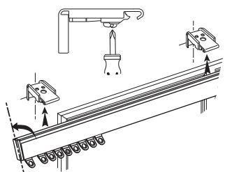
**12** With an equal number of glides located at each end of the track, angle the track with the glides forwards and up as shown. Offer the track up to the brackets and rest into place into the front of the brackets as shown in fig (i).
